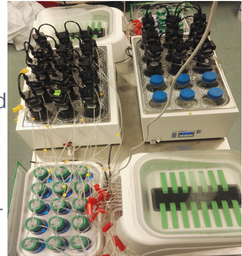
BMP equipment at Novia UAS in Technobothnia, Vasa, two units of AMPTS II, Bioprocess Control
