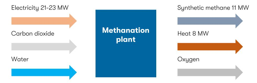
Synthetic methane is produced with microbes discovered in bogland, turning the carbon dioxide and hydrogen of the bioplant into synthetic methane. The technology was enabled by Q Power Oy.
